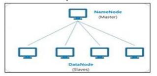
The first problem i.e. **Storing exponentially growing huge datasets** is solved using Hadoop as it divides a large file into small chunks and then stores them on different data nodes and these data files are also replicated so as to make the accessing of data easier. More no. of data nodes can be added as per the requirement.
