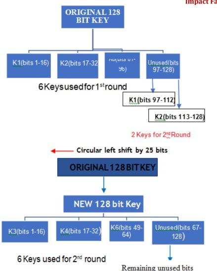
The new key is generated by shifting the bits of the original key circularly to the left afterevery round. As a result, the  $26^{\text{th}}$  bit of the original key shifts to the first position and becomes the first bit of the new key and the  $25^{\text{th}}$  bit of the original key moves to the last position and becomes  $128^{\text{th}}$  bit (after first shift) <sup>[12]</sup>.
